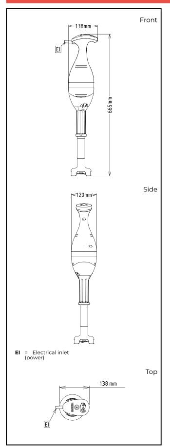
Electric Supply voltage: 220-240 V/1 ph/50/60 Hz **Electrical power max.:** 0.65 kW 0.65 kW **Total Watts:** Capacity: Capacity (up to): 80 Litre Key Information: External dimensions, Width: 138 mm External dimensions, 120 mm Depth: External dimensions, Height: 665 mm **Shipping weight:** 4.2 kg
